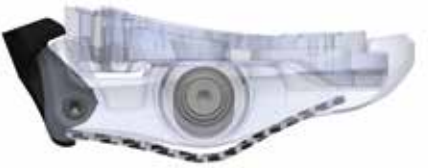
Deformation of the carbon blade during cleat release
